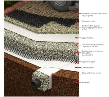
**3).** Please refer to tables 1 & 2 for guidelines to the depth of sub-base for specific design profile to suit different site needs. Please note - if a geogrid is omitted, 50% of the depth of sub-base needs to be added to calculated depth with a geogrid. For example, 100mm with geogrid would become 150mm without. For detailed guidance please contact our technical team.
