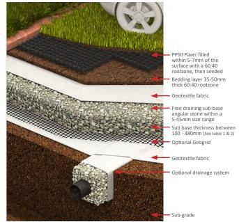
**3).** Please refer to tables 1 & 2 for guidelines to the depth of sub-base for specific design profiles to suit different site needs. Please note - if a geogrid is omitted, 50% of the depth of sub-base needs to be added to calculated depth with a geogrid. For example, 100mm with geogrid would become 150mm without. For detailed guidance, please contact our technical team.
